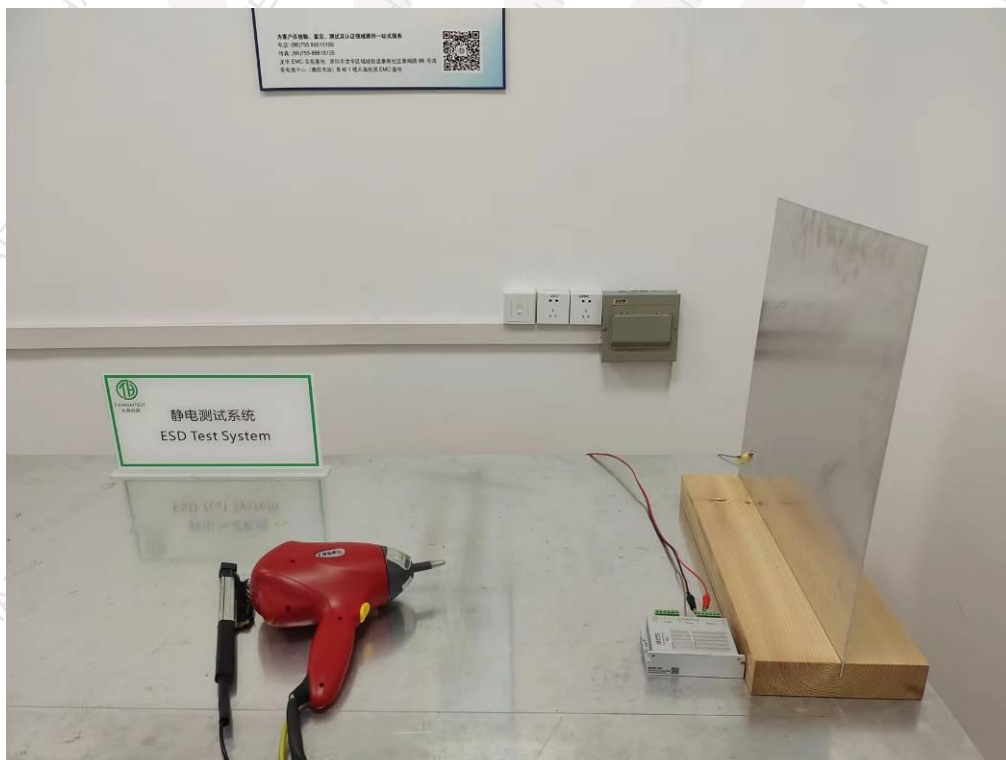
Photographs 2: Set-up for Electrostatic discharge (ESD)
